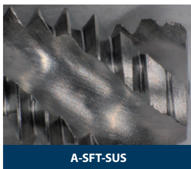
加工1,000孔后 Cutting edge after tapping 1,000 holes
