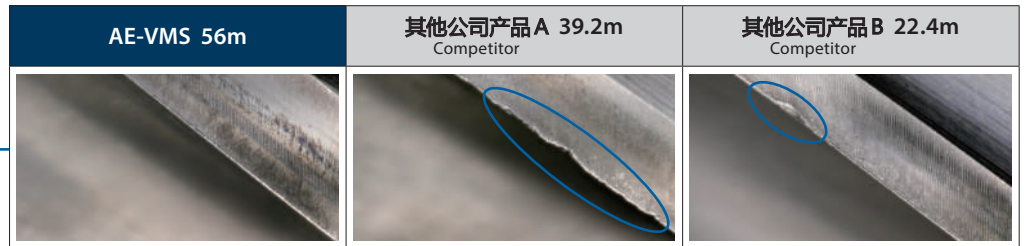
外周刃的磨损状态 Wear comparison of the peripheral cutting edge
