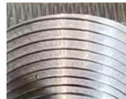
螺纹铣刀加工 Processing by thread mill
