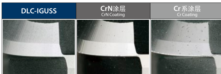
加工420m后球头部后刀面磨损状态 Wear condition of ball flank after milling 420m
