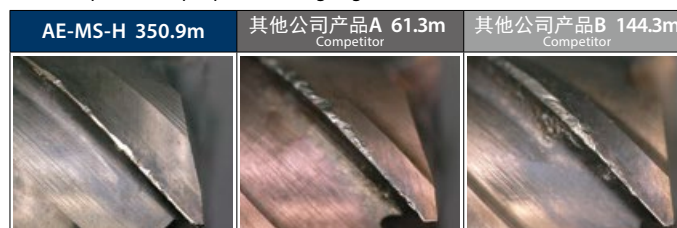
外周刃的磨损情况 Wear comparison for peripheral cutting edge
