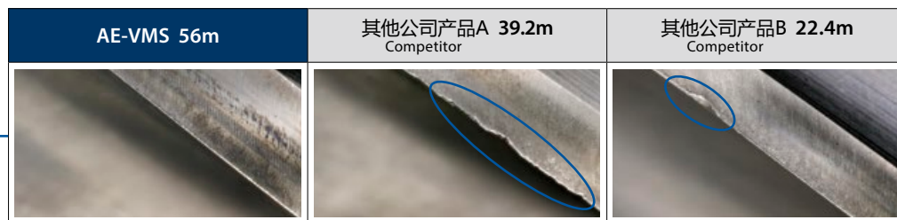
外周刃的磨损状态 Wear comparison of the peripheral cutting edge
