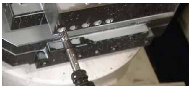
※挤压丝锥底孔加工请使用PXD 3D For tap drill hole of forming tap, 3D type should be used. (5D is not recommended)
