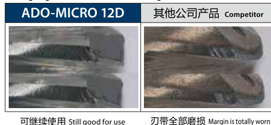
加工900孔后的刃尖状态 Cutting edge wear condition after drilling 900 holes
