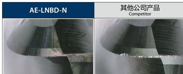
加工2,480m后的球头部后刀面磨损状态 Wearing condition of ball flank after milling 2,480m
