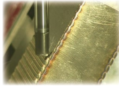
AM-CRE 加工190m后 After milling 190m
