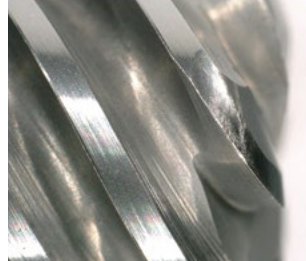
AM-CRE 加工190m后 After milling 190m
