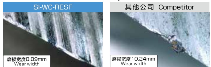
加工120分钟后的磨损宽度 Amount of wear after milling 120 minutes
