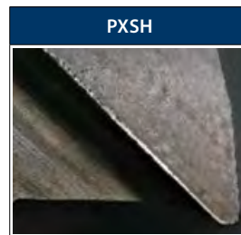
加工38.5m 后的刃尖损伤情况 Wear condition of the cutting edge after milling 38.5m
