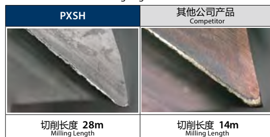
刃尖的损伤情况 Wear condition of the cutting edge
