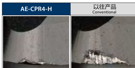
加工61.2m后的刃尖损伤状态 Wear comparison of the cutting edge after milling 61.2 m
