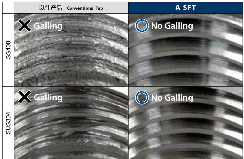
※内螺纹加工示意 Visual reference of internal threads. Result may differ based on actual machining condition.
